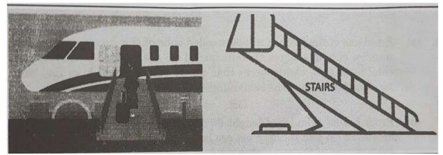
An air craft has a door sill at a height of 15 feet above the ground. A stair car is placed at a horizontal distance of 15 feet from the plane.
